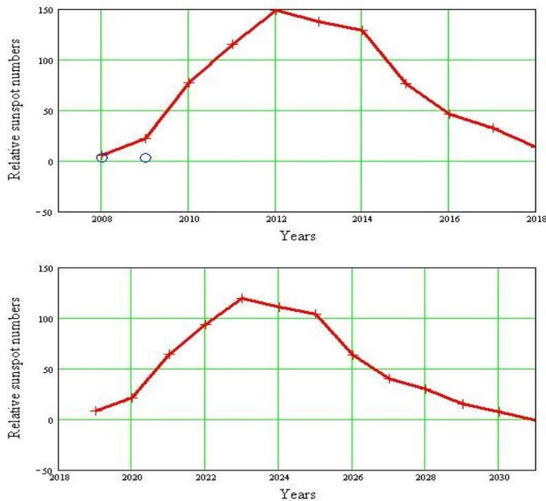
Fig. 4 – The cycles 24 and 25 activity level forecast: crosses represent the predicted values and circles represent the observed values for 2008 and 2009.
