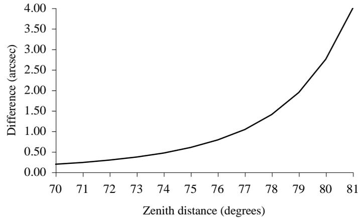
Fig.2 – Difference of the refraction values for the latitude of 45°.
