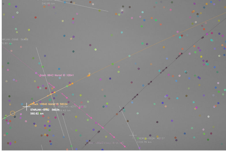
Fig. 2 – Image generated during real time operation of the wide FOV sky surveillance system, May 11, 2024. The colored trajectories are detected tracklets in image coordinates, and the white trajectories are the predicted satellite trajectories based on orbital information. In this image, we can see that the Starlink 5782 satellite's actual position seems to fall behind its predicted position (white cross).
