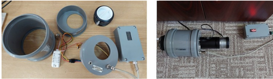
Fig. 6 – The component parts of the sealed enclosure(left). Mounted sealed enclosure (right).
