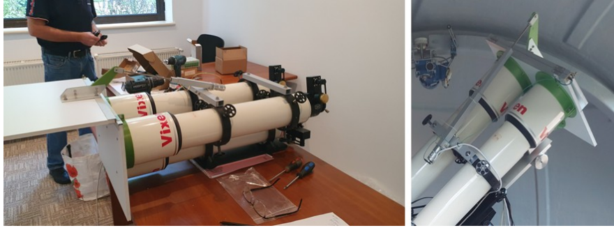
Fig. 4 – The hinged cover fixed to the three telescopes by plastic rings made by 3D printing and operated by an actuator.
