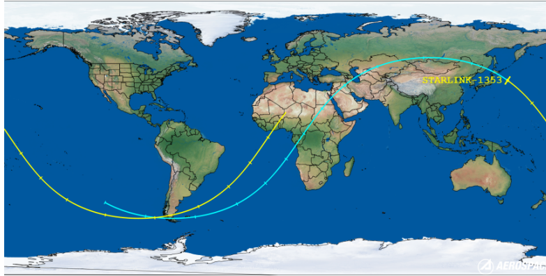
Fig. 1 – Prediction Ground Track for Starlink-1353 satellite (Aerospace, 2023)
