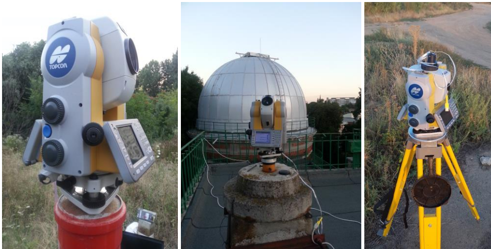
Fig. 3 – Three stationed astro-geodetic points: left figure, HTL (pilaster, forced centering); center figure, AIRA (pilaster, forced centering) and right figure, the E station (stationed on the tripod of the total station).
