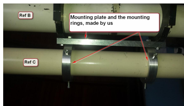
Fig. 7 – Installation of Ref C on the equatorial mount and on the mounting rings of Ref B.
