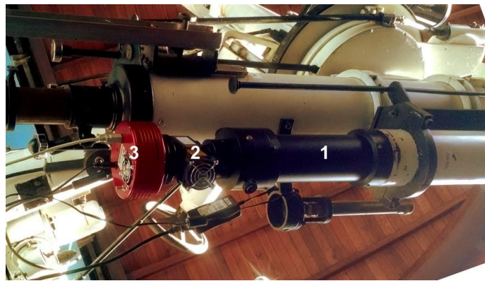
Fig. 1 – Optical scheme and photo of Ref B before upgrade: (1) TZ2 adapter, (2) Ha filter, (3) ATIK 4000 CCD.
