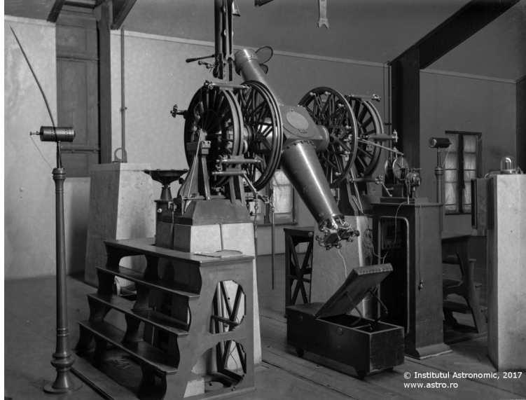
Fig. 5 – Gautier-Prin telescope during usage in the Meridian Hall of Bucharest Observatory (1920's photo).
