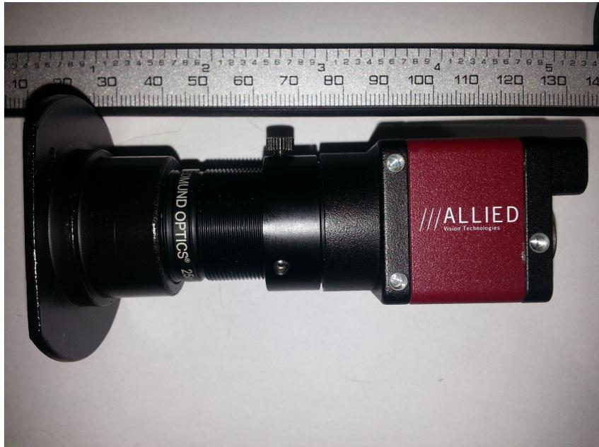
Fig. 5 – The realized mount made by Duramid (left), the EO micro-objective (center) and micro-CCD camera Guppy Pro F-046 (right).
