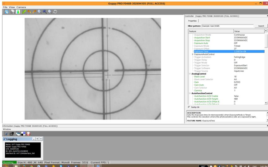
Fig. 6 – A daytime test image obtained in laboratory on a calibration target, with Guppy Pro F-046 B&W mounted on Topcon MS05AX using the AVT Vimba Viewer software.
