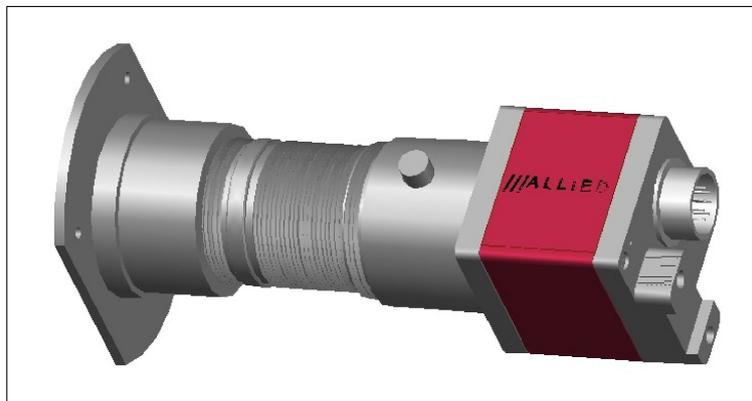
Fig. 4 – The 3D project of the mount that couples the CCD micro-camera to the optical system of the total station.
