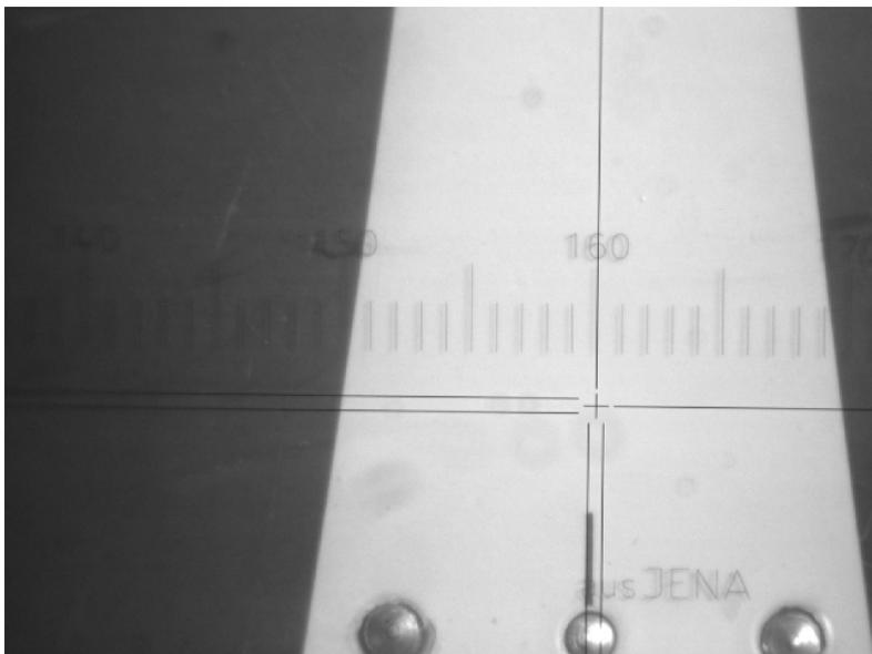
Fig. 8 – A daytime test image obtained in laboratory on a millimeter divided calibration ruler, with Guppy Pro F-046 B&W mounted on Topcon MS05AX.
