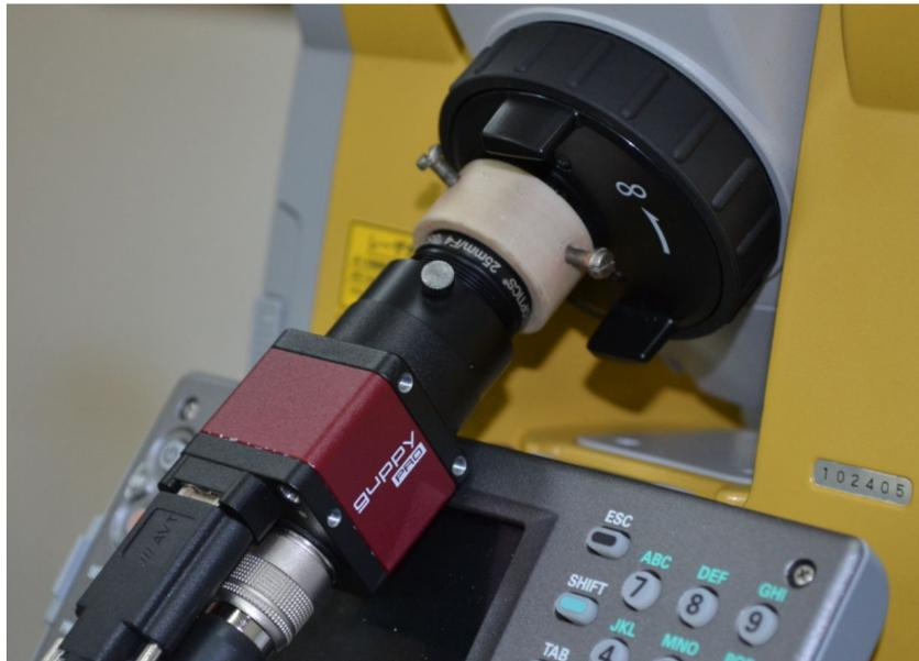
Fig. 2 – The handcrafted mount prototype, made of plastic.
